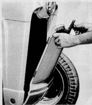
Figure 27 Opening Radiator Grille
