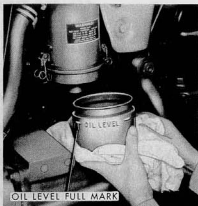
Figure 19 Checking the Air Cleaner Oil Level
